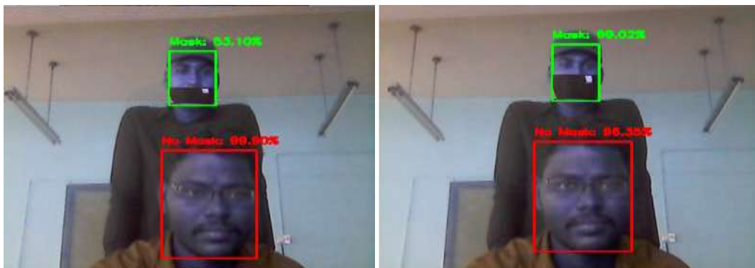
Figure 15 Screenshots of No Mask, Partial Mask and Full Mask Detection with two persons using CNN
