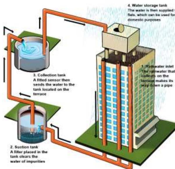
Figure 5: rain water harvesting
