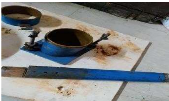
Standard Proctor Compaction Test
