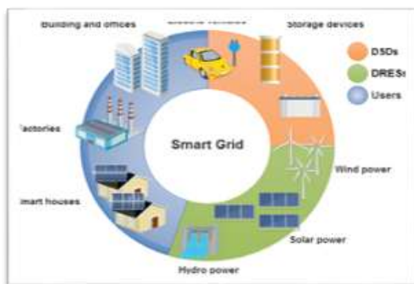
Fig 6: Smart grid components
